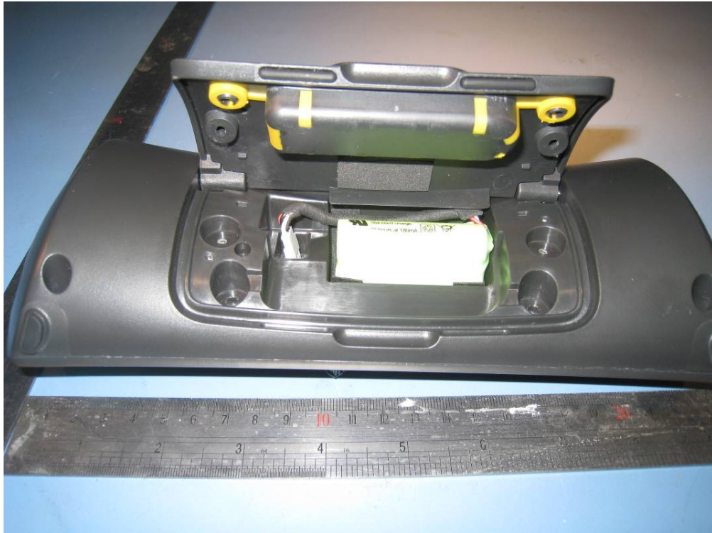
Fig. 1: Rear view of battery storage location
