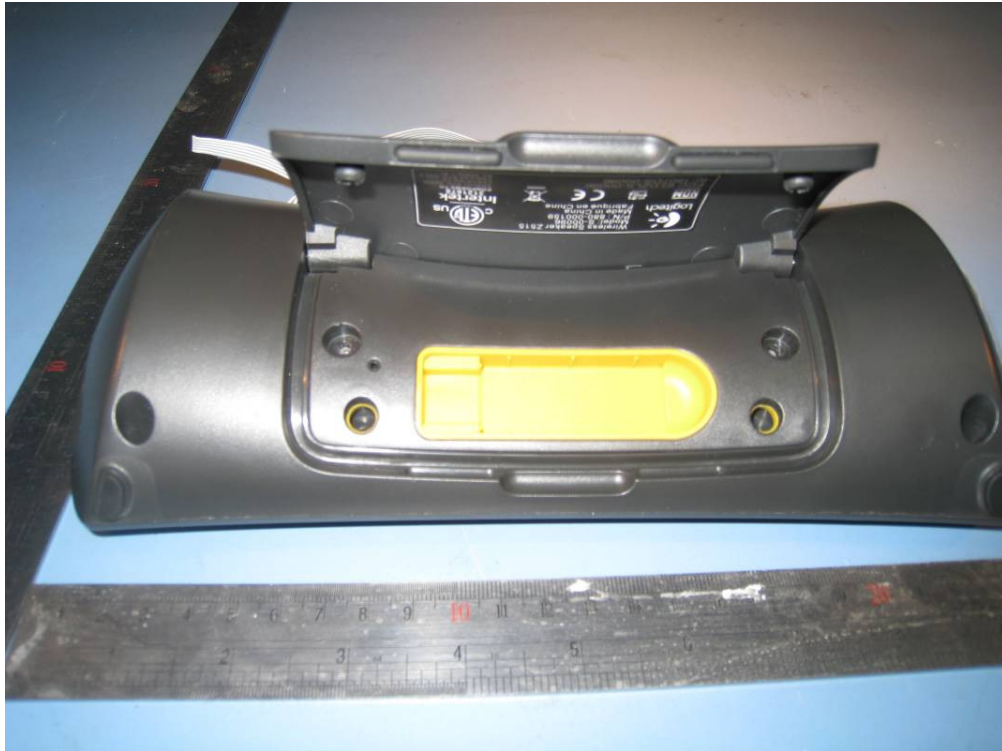
Fig. 5: Rear view with tongue storage compartment
