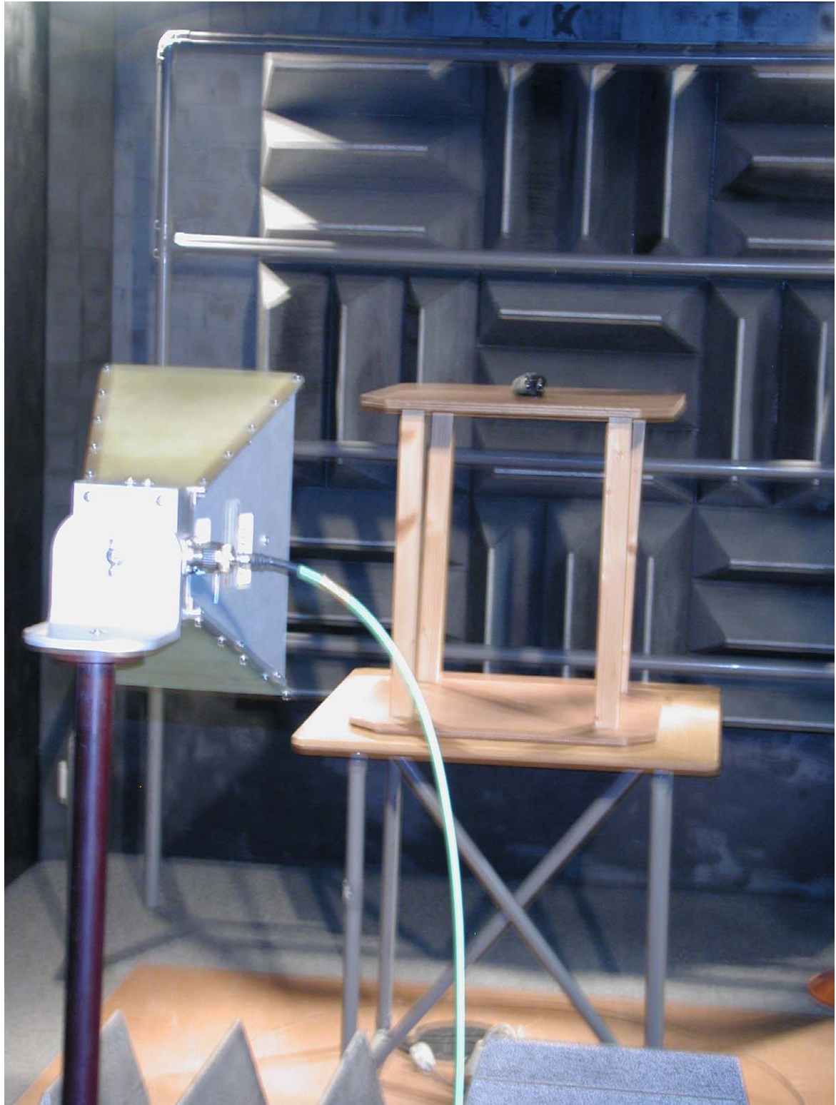
Photograph 2: Test setup radiated emissions (exploratory >1000 MHz)
