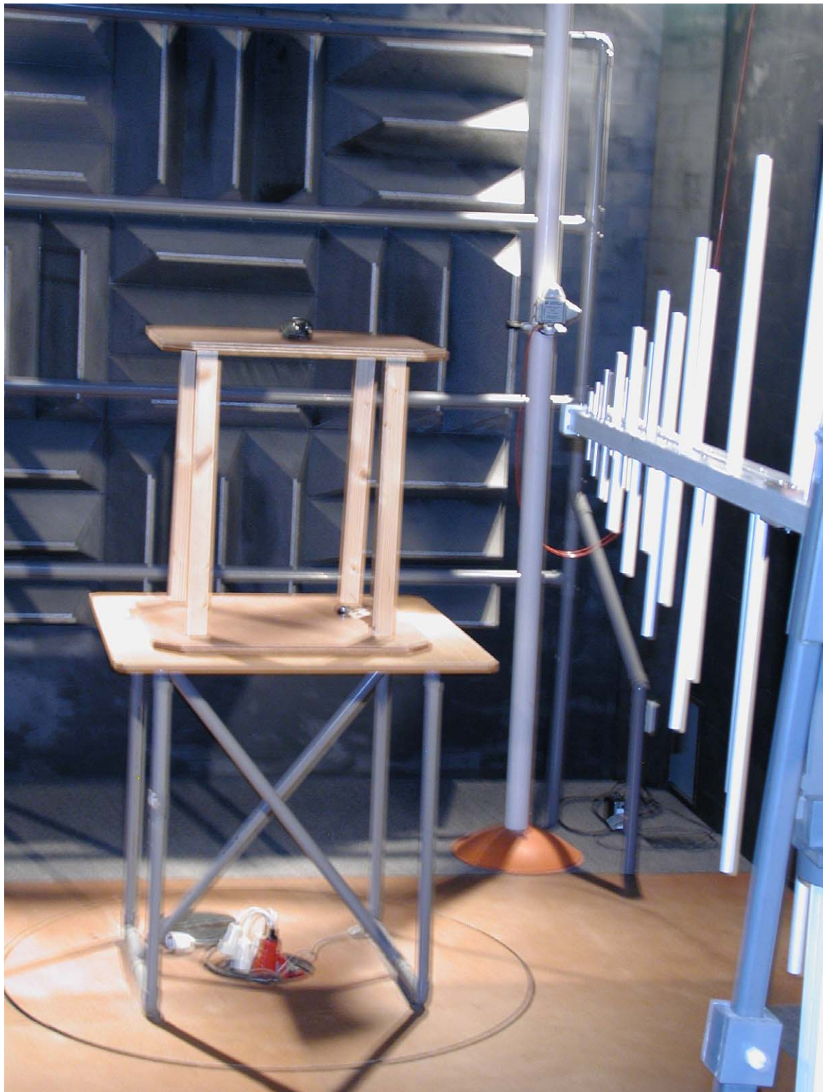
Photograph 1: Test setup radiated emissions (exploratory <1000 MHz)
