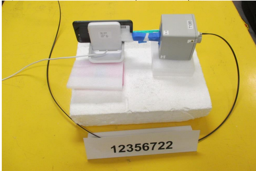
S1, RF EXPOSURE SETUP PHOTO (HORIZONTAL)
