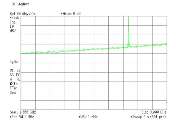
Note: The peak shown in the plot is the carrier frequency.
