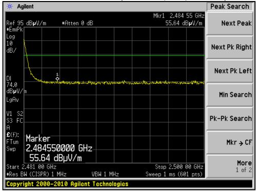
\* The average value is Average value = peak reading + 20log(duty cycle). And it meets the requirement of limit.
