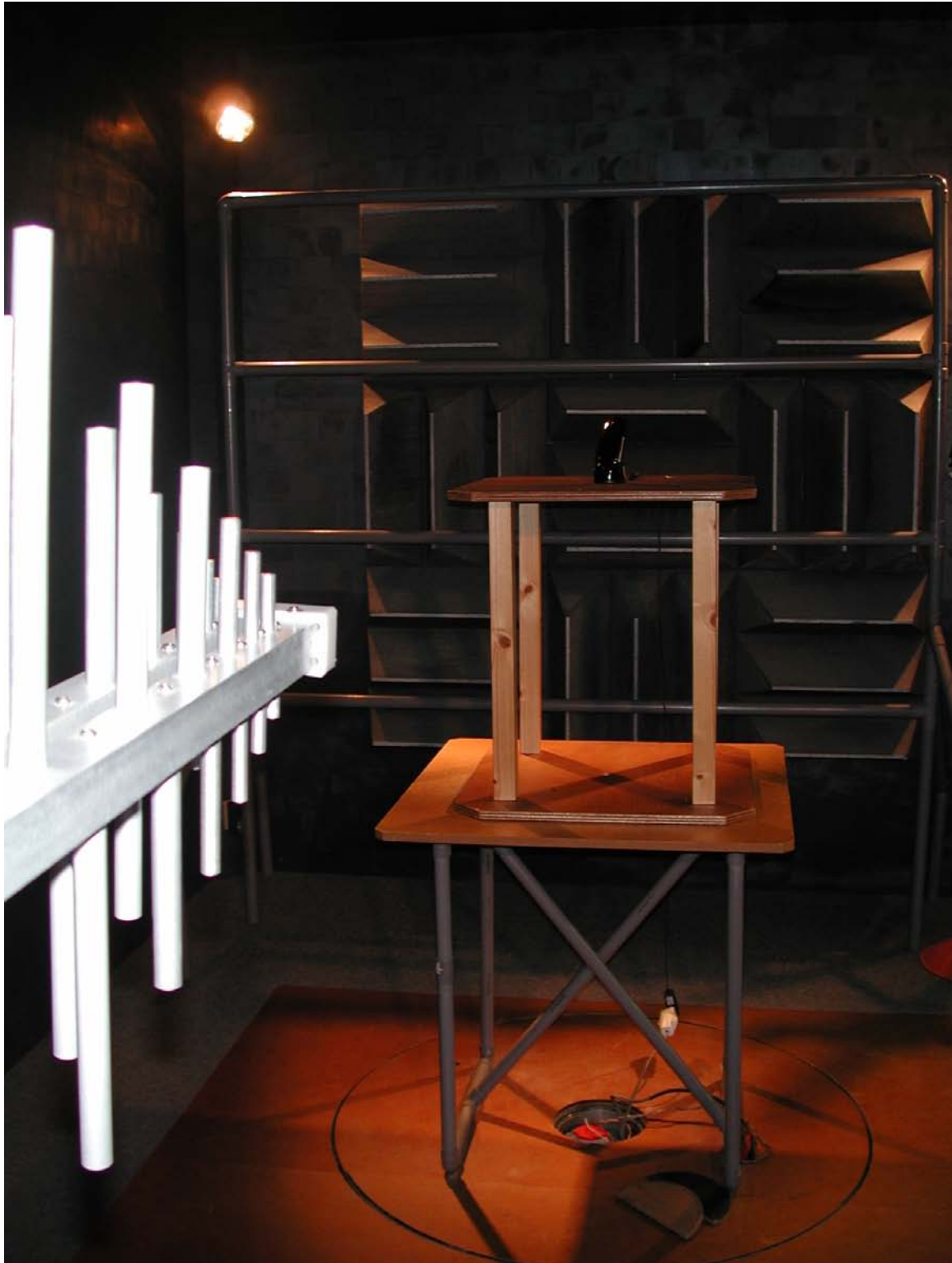
Photograph 1: Test setup exploratory radiated emissions up to 1000 MHz
