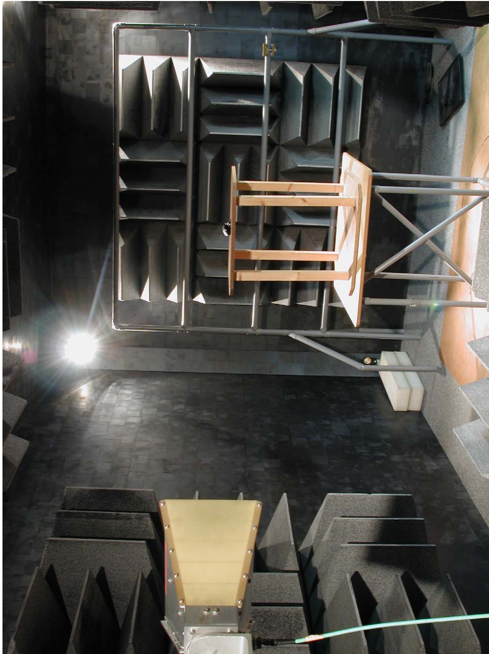
Photograph 2: Test setup radiated emissions > 1000 MHz
