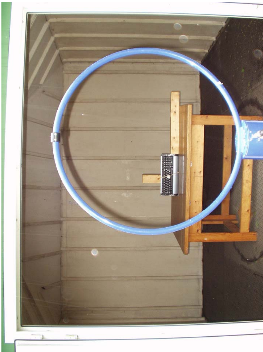
Photograph 1: Test setup OATS < 30 MHz
