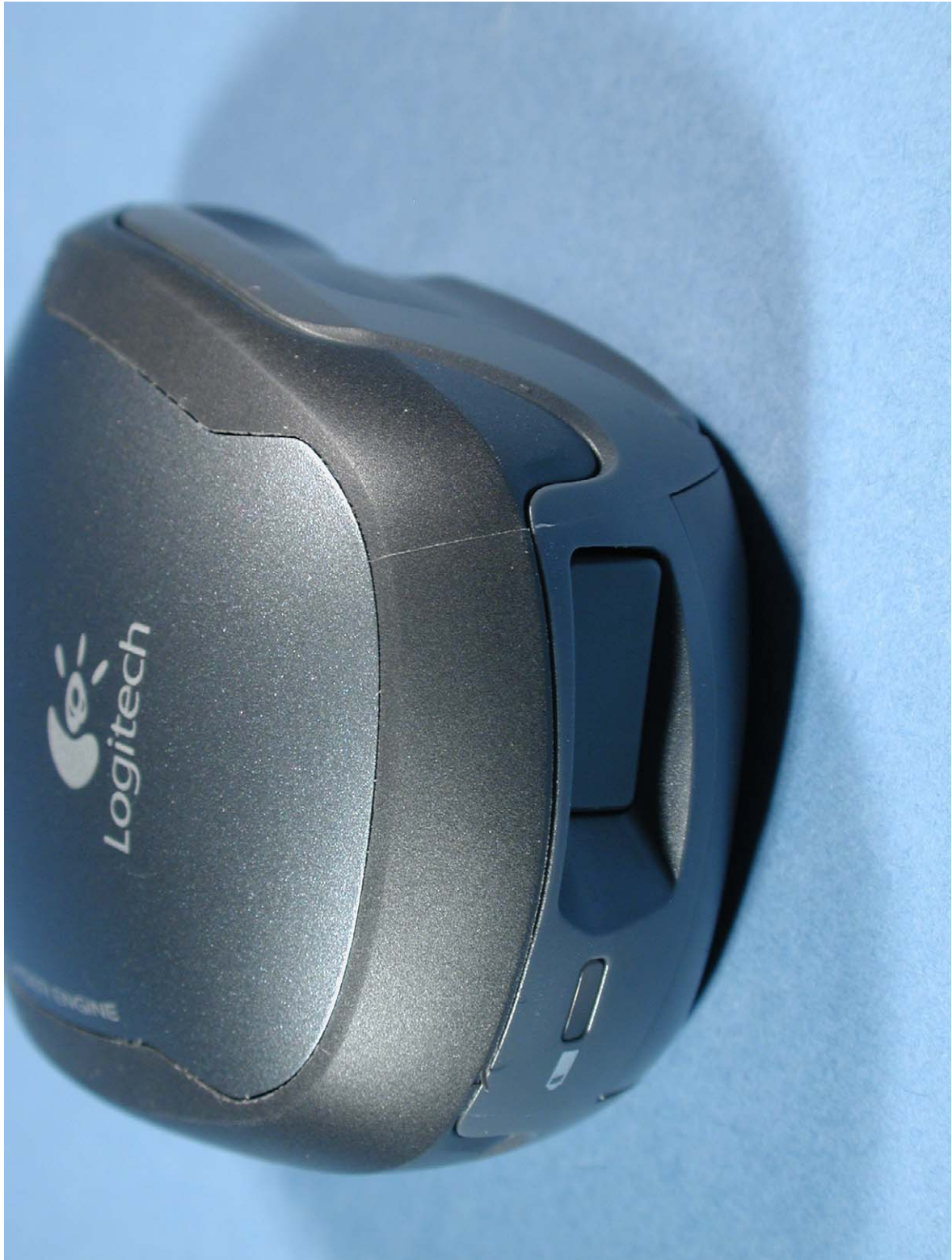
Photograph 3: M-RBL117 battery LED and receiver storage
