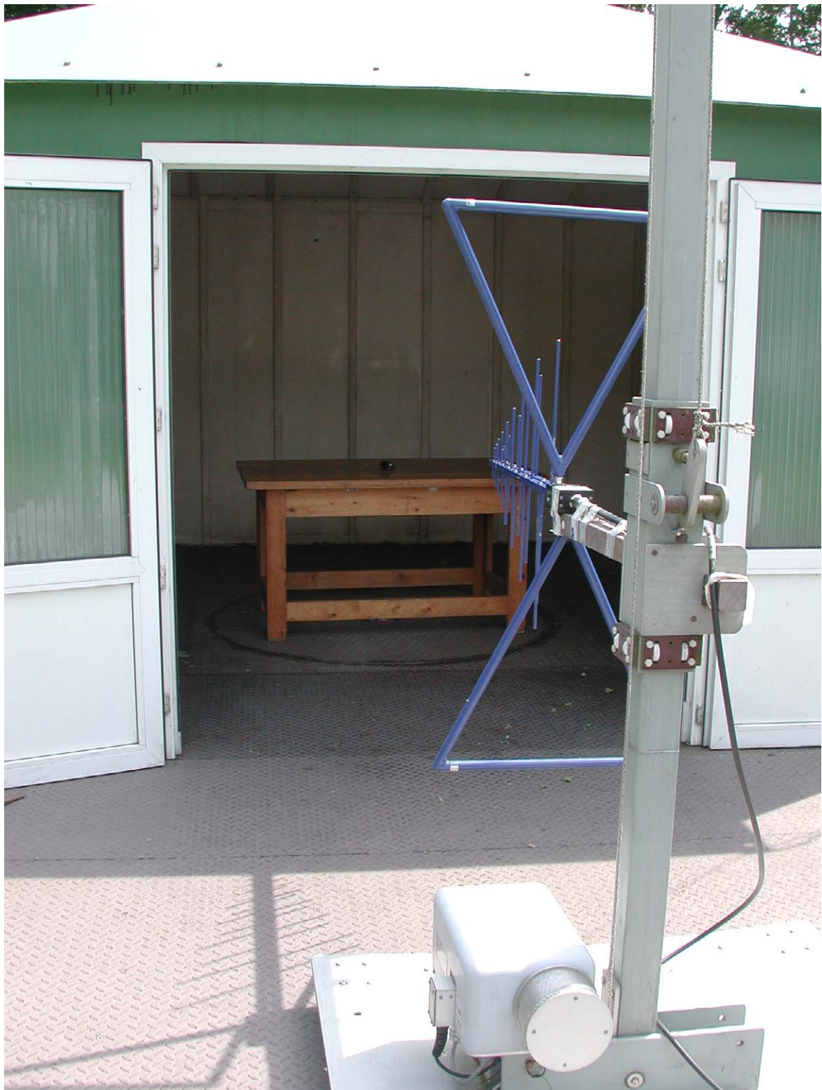
Photograph 15: Test setup OATS > 30 MHz
