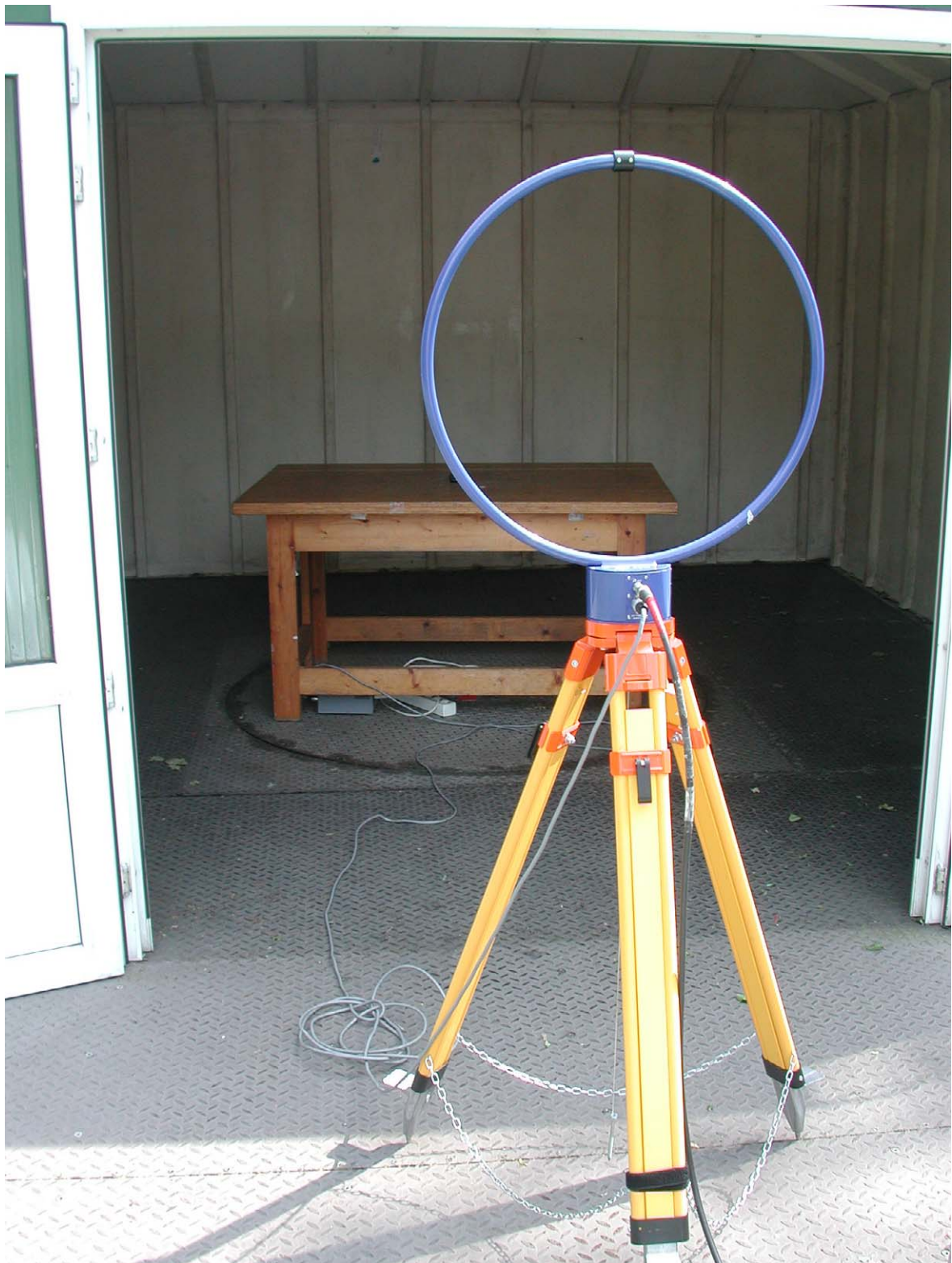
Photograph 14: Test setup OATS < 30 MHz
