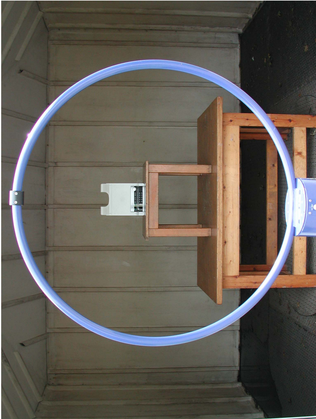
Photograph page 4: Test set up Y-RX43: magnetic radiated emissions (Y-POS)
