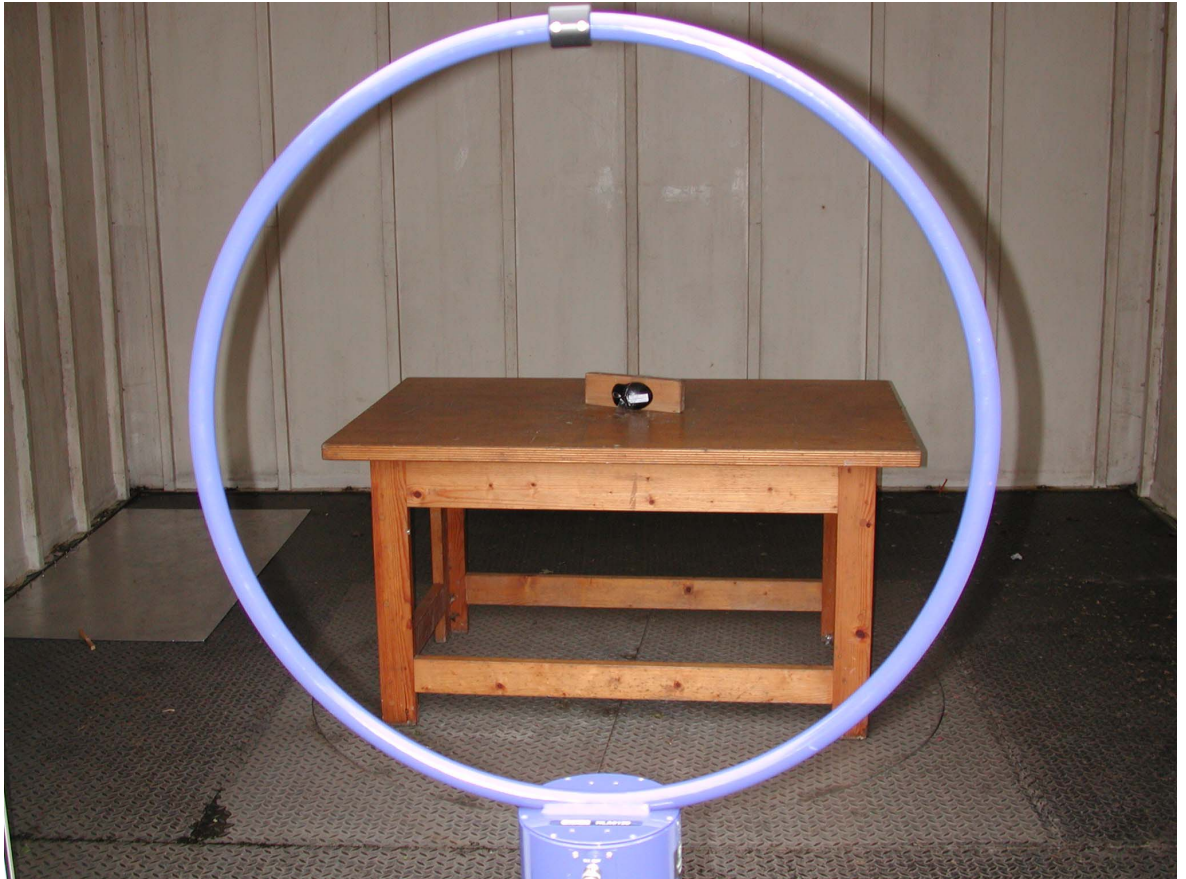
Photograph 2: Test set up: magnetic radiated emissions at 3 m distance (EUT in X plane)
