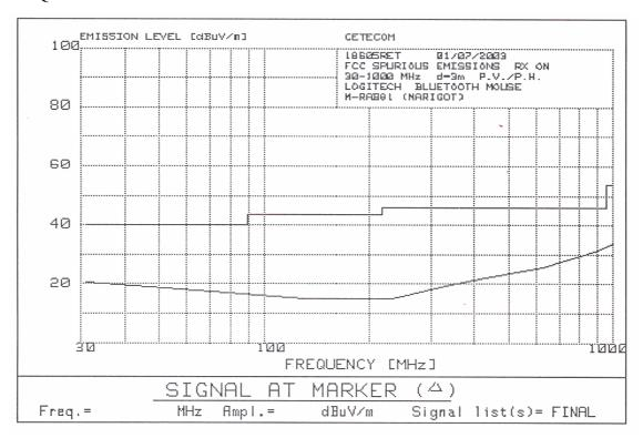
Resolution bandwidth= 100 kHz Video bandwidth= 100 kHz
