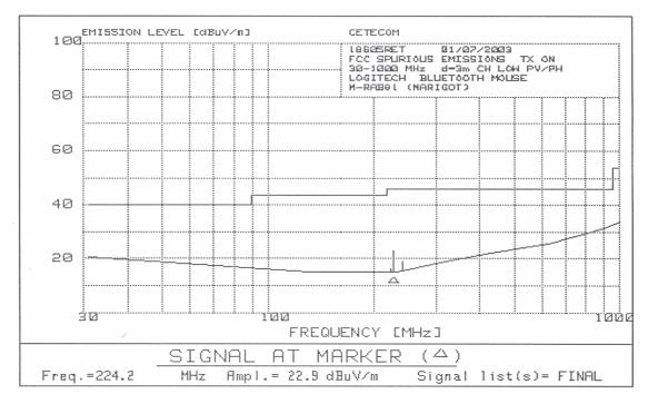
Resolution bandwidth = 100 kHz. Video bandwidth = 100 kHz.
