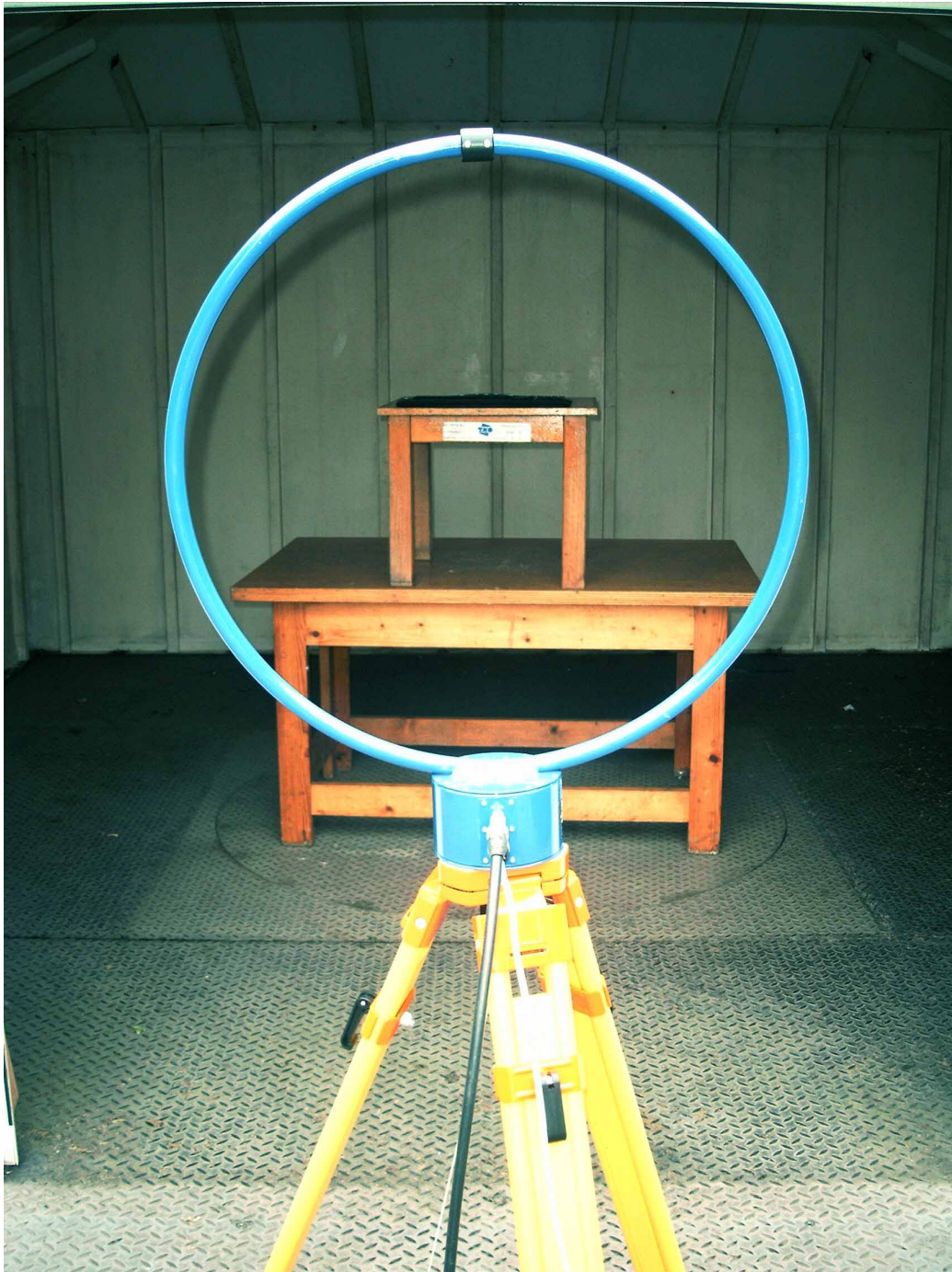
Photograph page 5: Test set up Y-RQ52: magnetic radiated emissions (X-POS)
