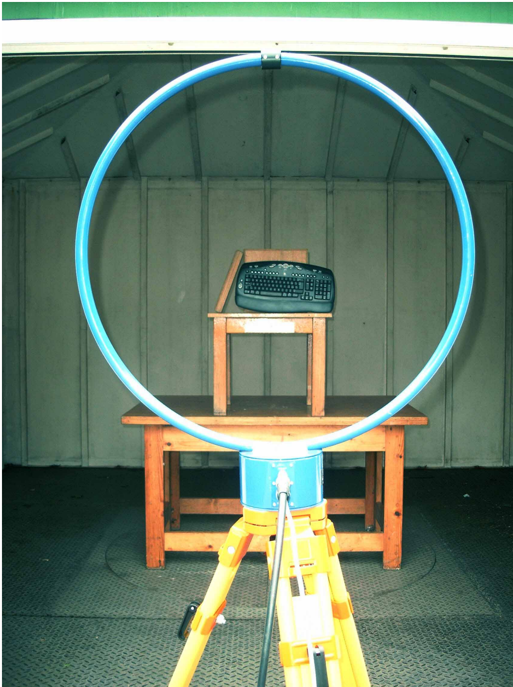
Photograph page 6: Test set up Y-RQ52: magnetic radiated emissions (Y-POS)
