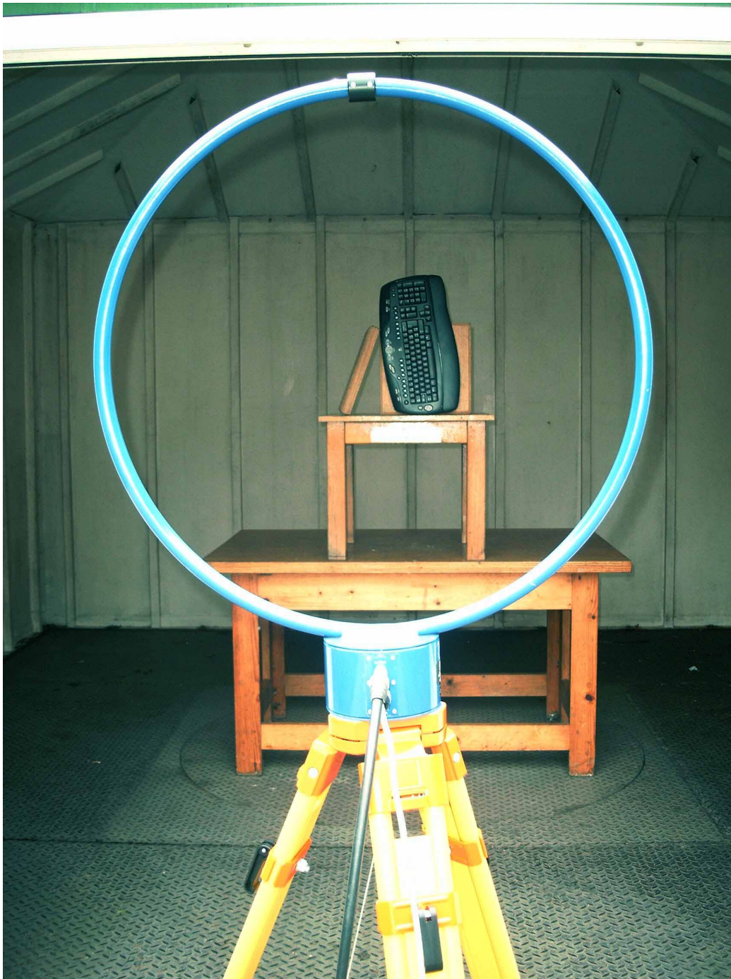
Photograph page 7: Test set up Y-RQ52: magnetic radiated emissions (Z-POS)
