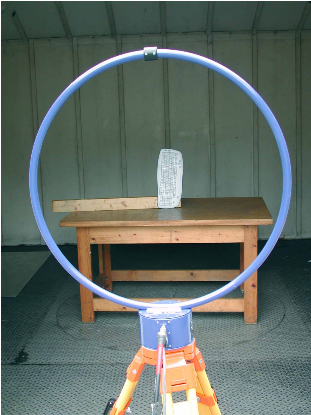
Photograph page 9: Test set up Y-RR57: magnetic radiated emissions (Z-POS)
