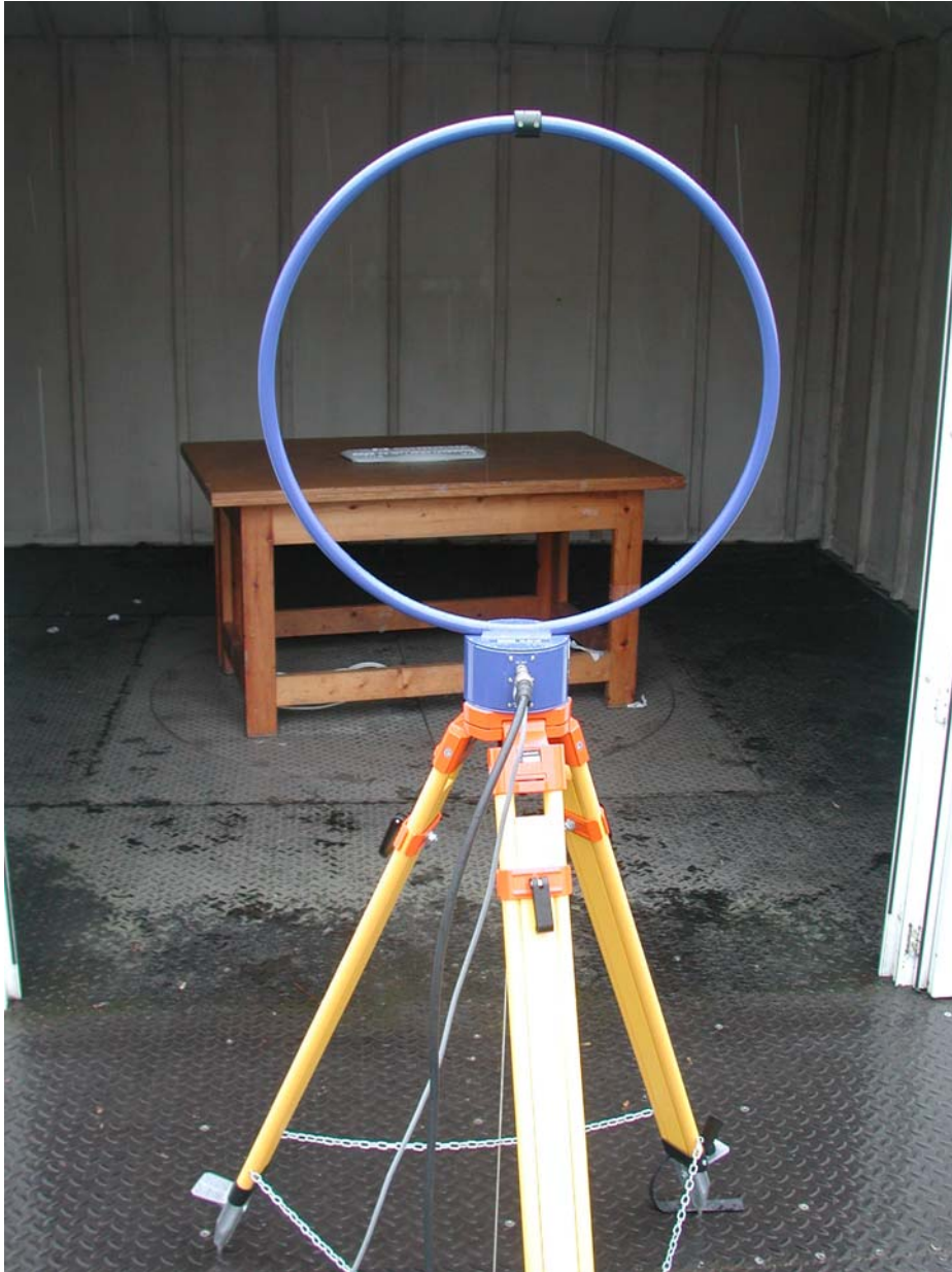
Photograph 2: Test set up: magnetic radiated emissions at 3 m distance (EUT in X plane)
