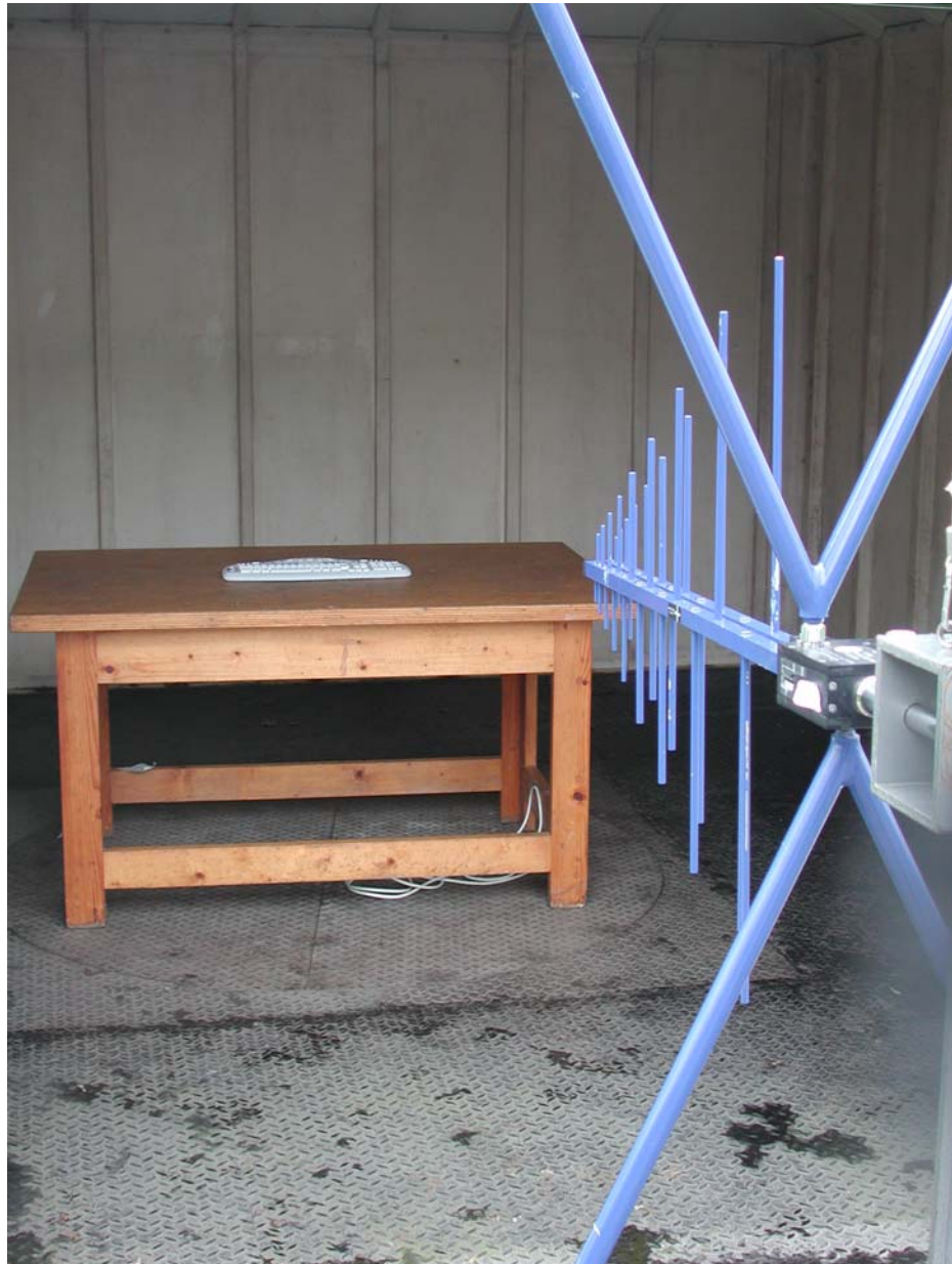
Photograph 3: Test set up: radiated emissions above 30 MHz at 3 m distance
