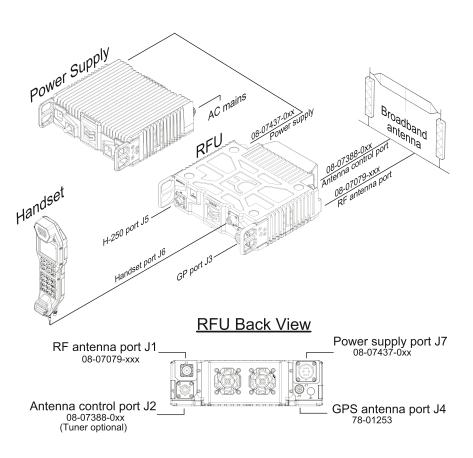
NOTE: A range of ancillary equipment may be connected to the Sentry-H transceiver using the H-250 port and, GP port connectors at the front of the RFU.
