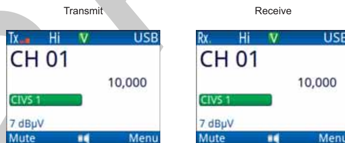
Figure 54: Channel screen showing transmit/receive status for CIVS voice scrambler
