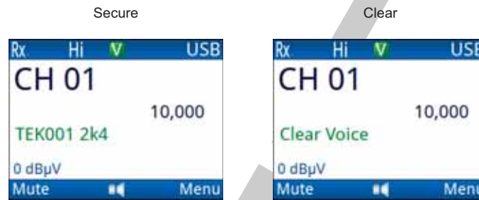
Figure 57: Channel screen showing secure/clear status for AES-256 digital voice encryption
