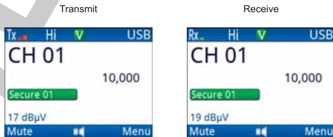
Figure 56: Channel screen showing transmit/receive status for CES-128 voice encryption
