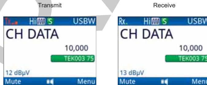
Figure 62: Channel screen showing transmit/receive status for AES-256 digital data
