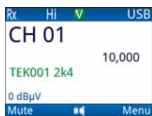
Figure 59: Channel screen showing AES-256 secure key and data rate
