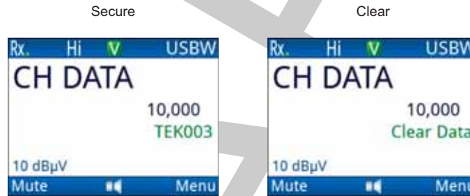
Figure 61: Channel screen showing secure/clear status for AES-256 digital data
