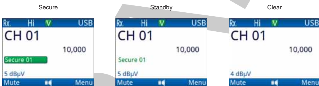
Figure 56: Channel screen showing transmit/receive status for CES-128 voice encryption
