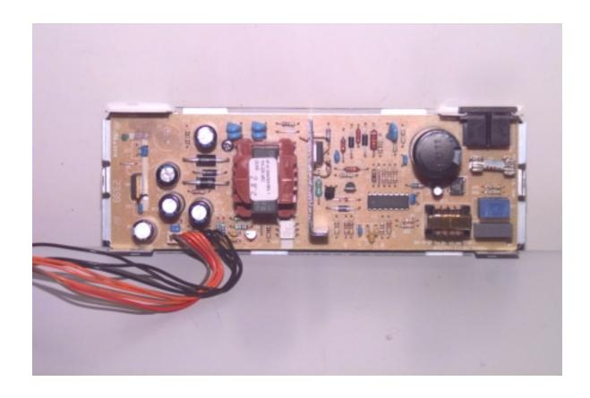
Fig. 8.6 Power Supply Unit P.W.A. - Foil side
