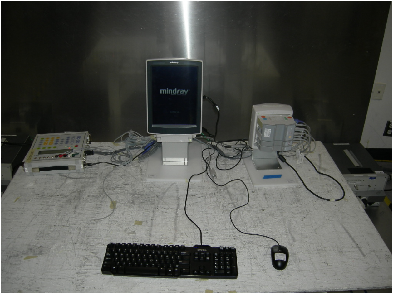
Figure 3: AC Power Line Conducted Emissions - V12
