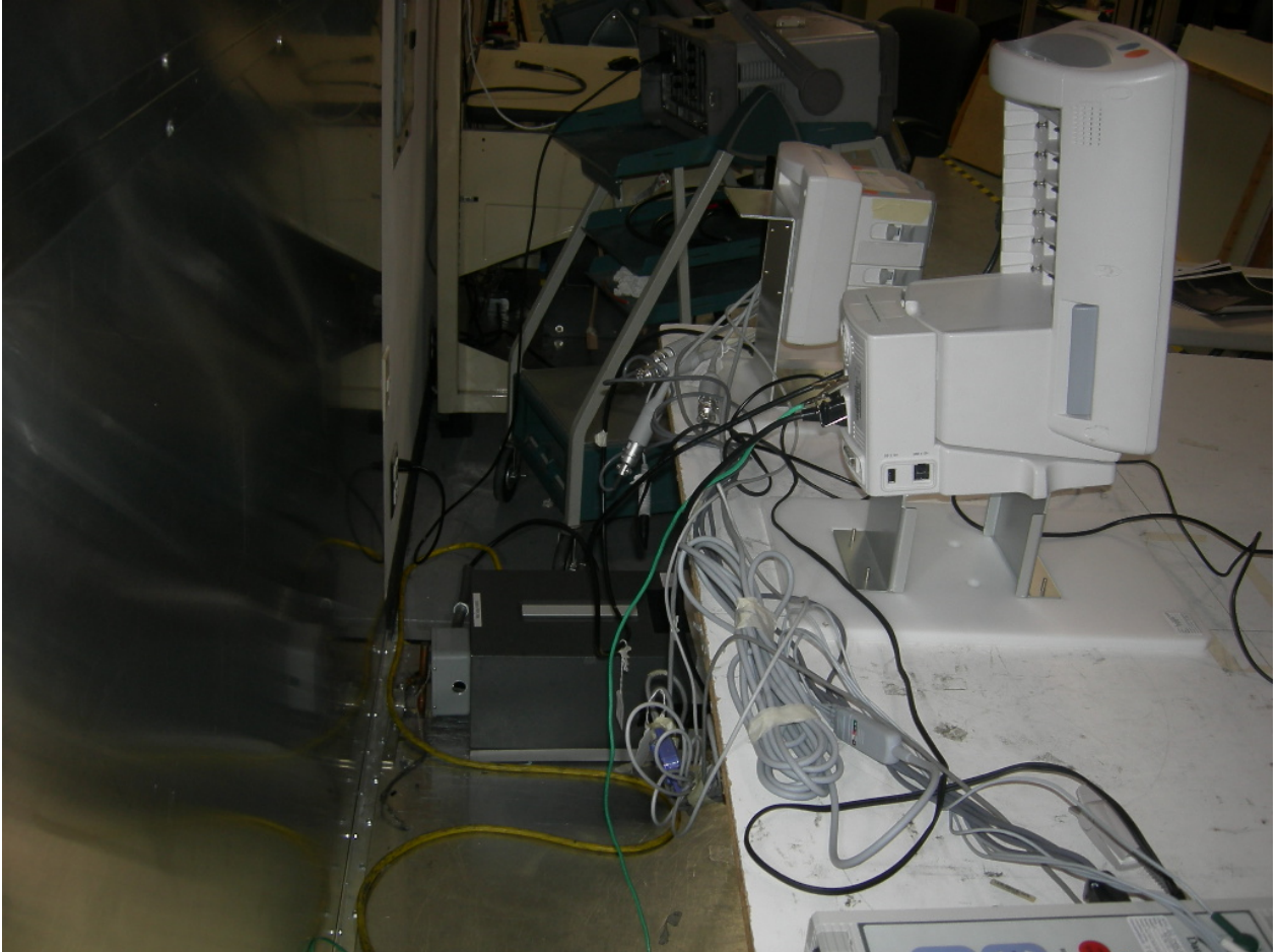
Figure 4: AC Power Line Conducted Emissions - V12
