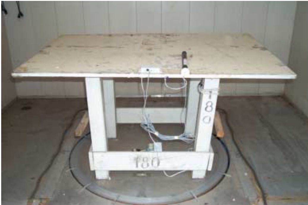
Figure 3.1 Radiated Test Setup
