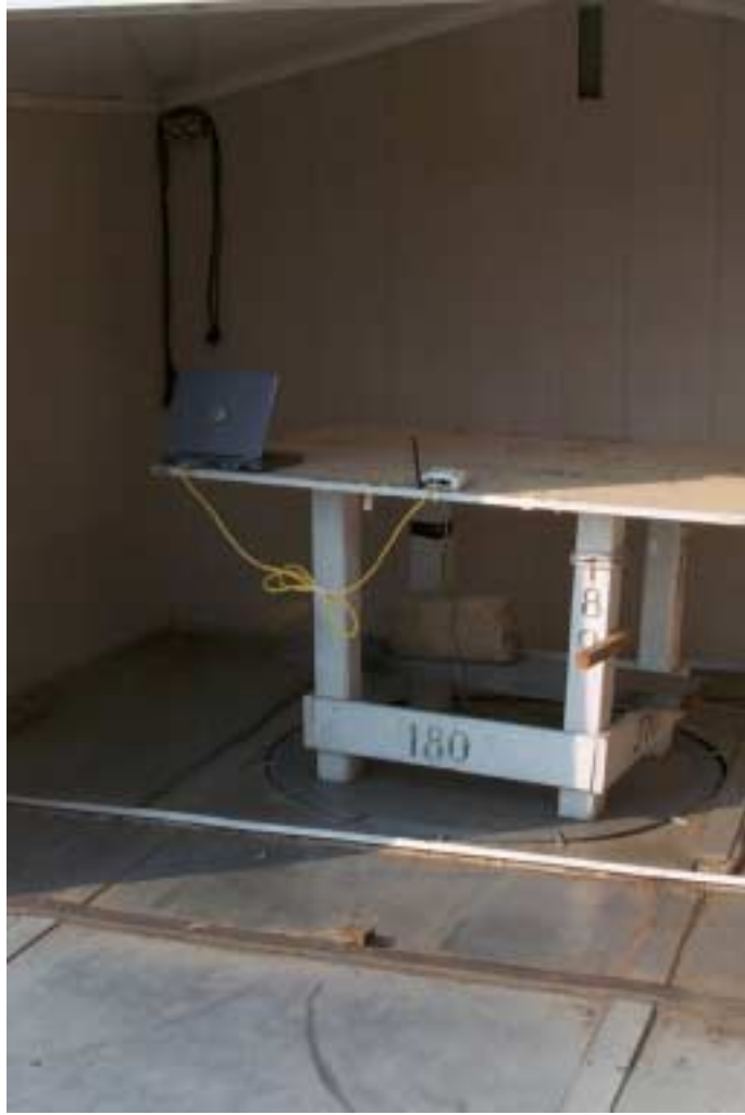
Figure 3.3 Radiated Test Setup, position 3-Z
