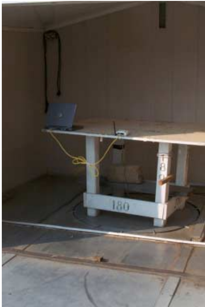
Figure 3.3 Radiated Test Setup, position 3-Z
