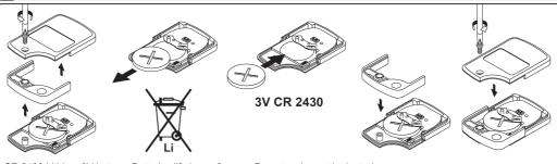
CR 2430 Lithium 3V battery. Batteries lifetime: ±2 years. Do not recharge the batteries.
