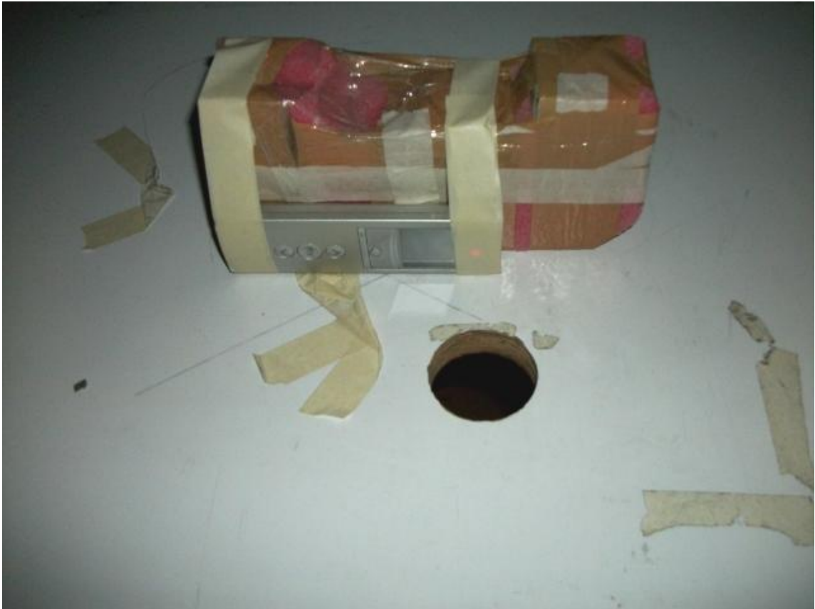
Figure 3.2 Radiated Test Setup, position 3-Y
