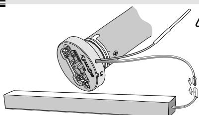
**⚠** Do not unplug the battery when the motor works.
