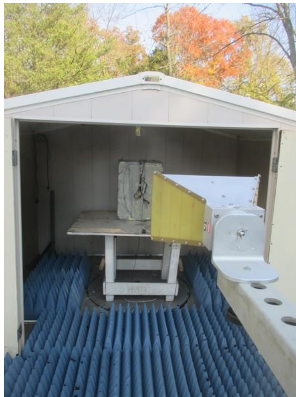
Figure 3.1 Radiated Test Setup
