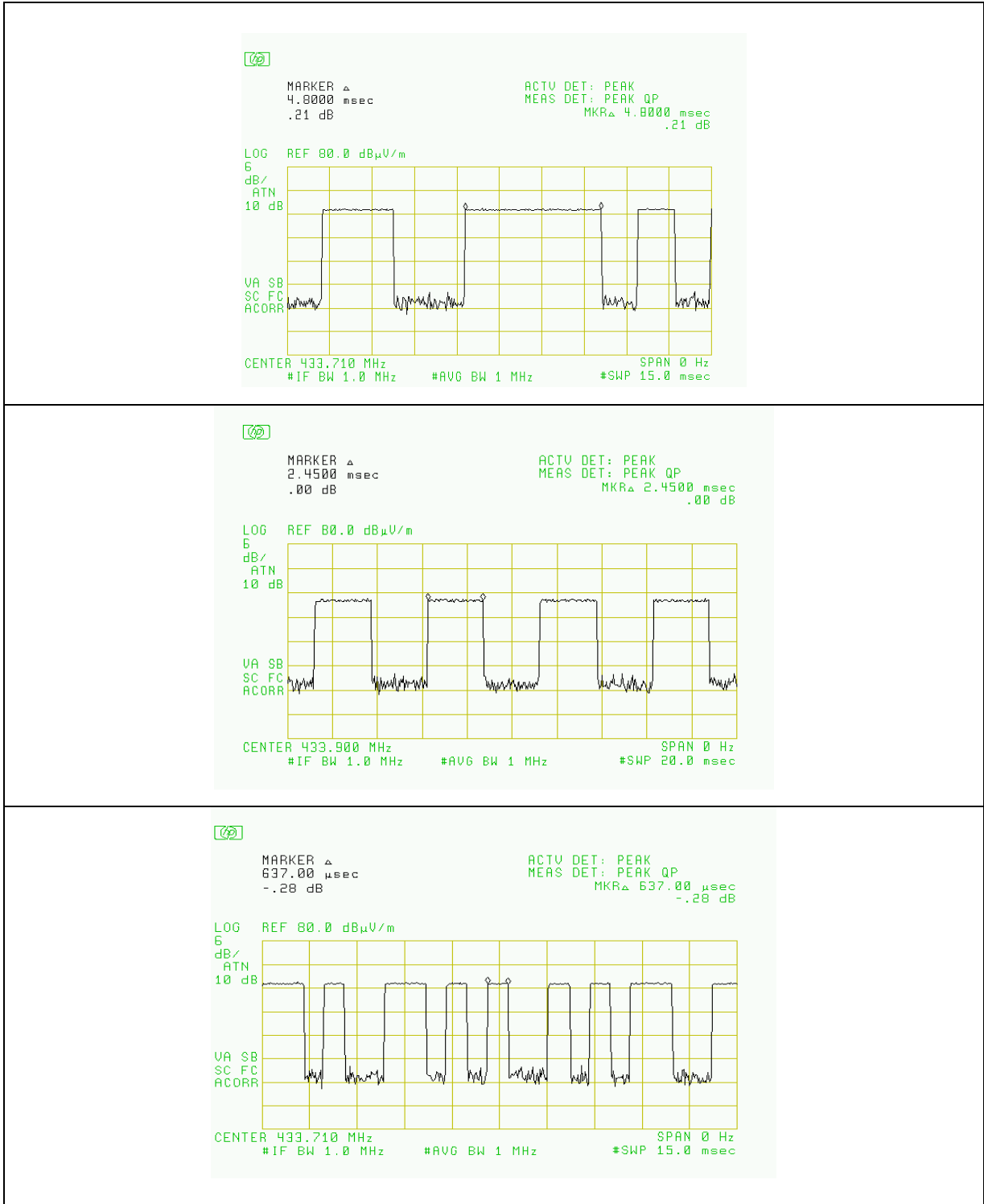
Figure 6.2 Pulse Train Timing
