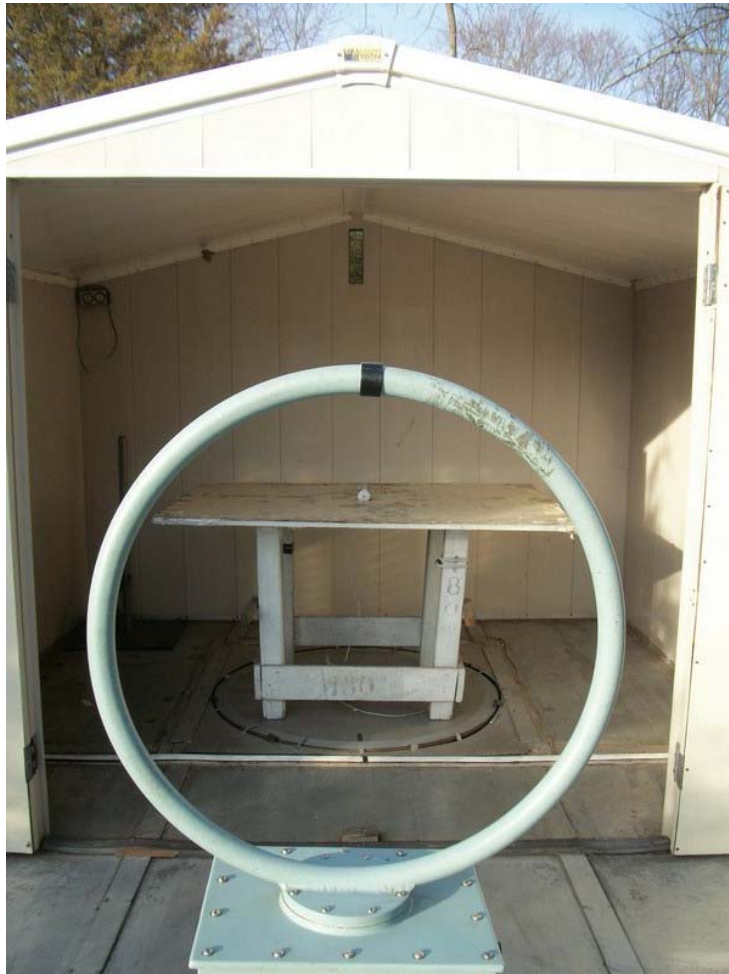
Figure 3.1 Radiated Test Setup
