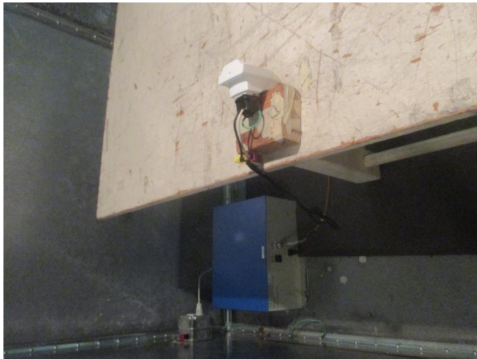
Figure 3.2 Conducted Test Setup
