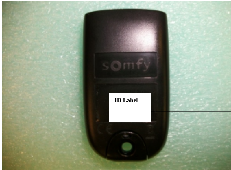
Figure 2.2 ID Label Location
