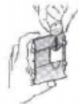
5. Replace the battery with the correct polarity and once again press the Inis RT switch button. The motor will JOG briefly to confirm programming.
