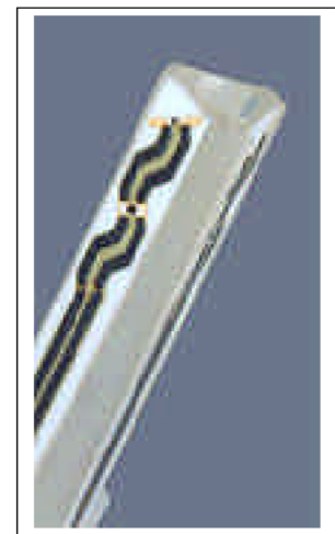
Inside view of ET3DV6 E-field Probe
