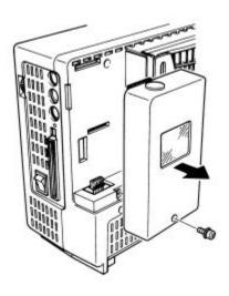
The transmission module housing is located at the upper left of the DS-5100 as viewed from the rear.
