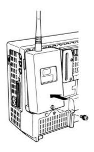
Place the cover back in its original position while at the same time inserting the antenna into the antenna hole. Replace the cover onto the DS-5100 by replacing the screw at the bottom.
