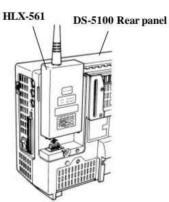
Connect the cable from the bottom of the module housing to the connector at the bottom of the HLX-561. Remove the cap which covers the antenna hole in the top of HLX-561 transmission module housing cover. Place the HLX-561 into the housing, taking care not to jam the cable in the inside.
