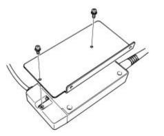
Attach the optional mounting fixture onto the HLX-561 with two accessory screws (M2.6 x 6).
