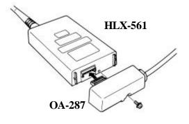
Connect the optional OA-287 adapter to the HLX-561, connector to connector. Attach the adapter to the HLX-561 with the accessory screw (M2.6 x 8).
