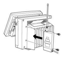
Attach the assembly consisting of the HLX-561, OA-287 and mounting fixture, to the DS-5300 with the two accessory screws (M3 x 6).
