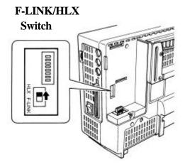
The F-LINK / HLX switch is now accessible. Switch to the HLX position to effect internal communication (Setting this switch to the HLX position disables the external F-LINK connector.)
