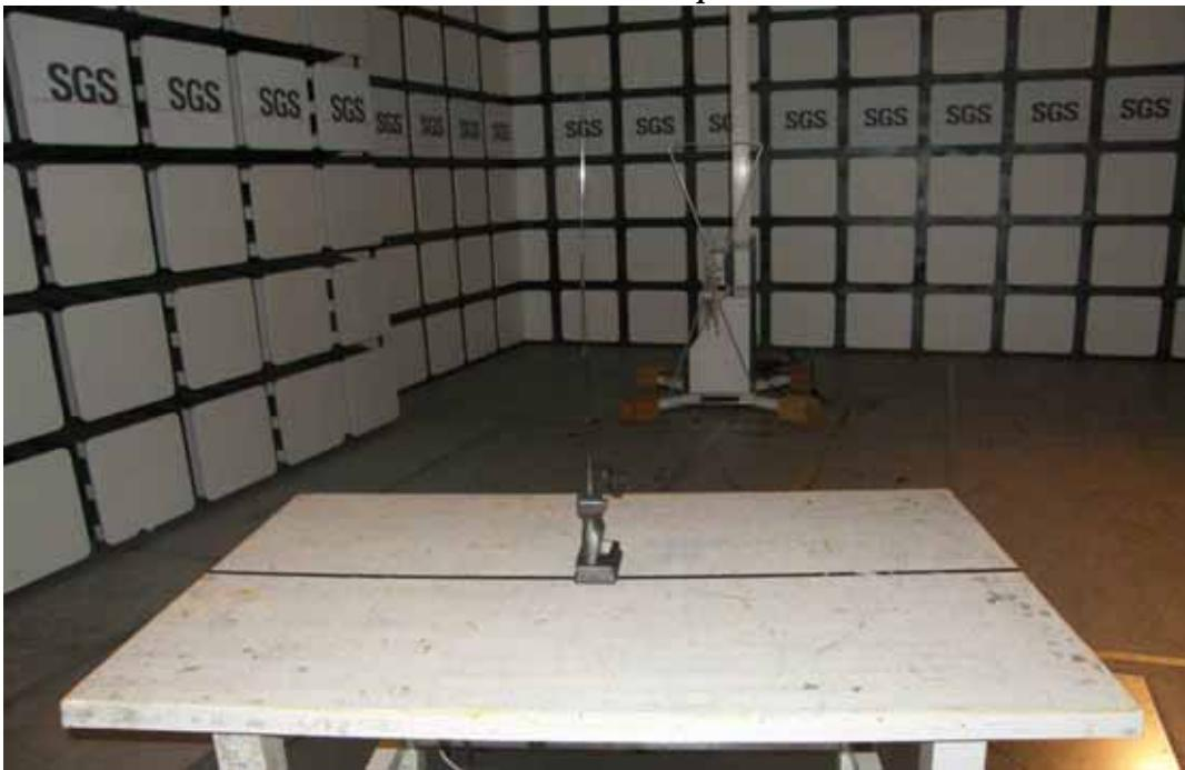
*Radiated Emission Setup Photo (EUT only)*
