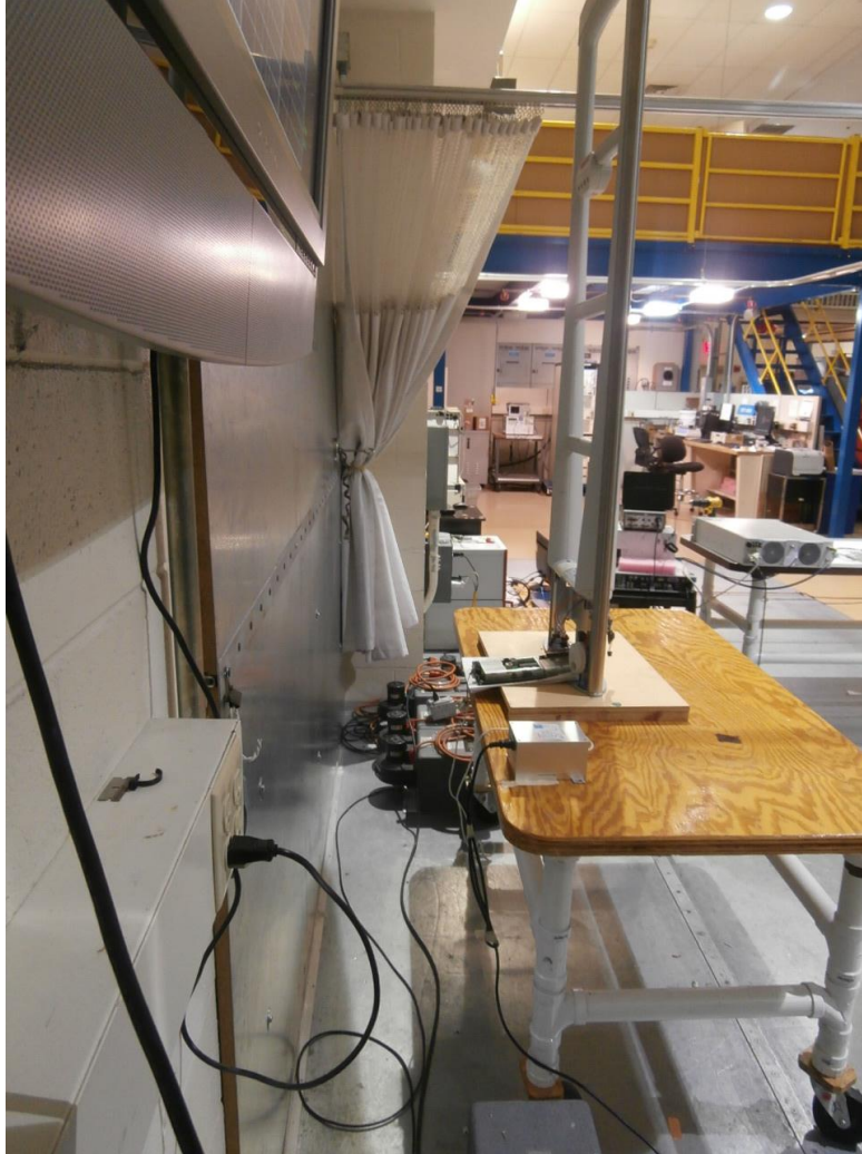
LINE CONDUCTED EMISSION (BACK – WITH ANTENNA)
