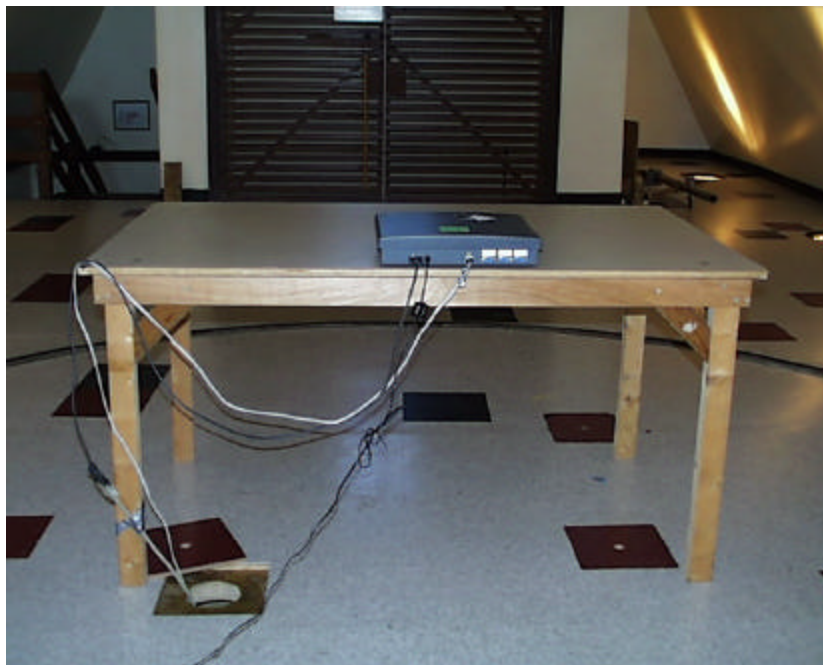
Photo 3 – Radiated Emissions Test Setup – Rear View
