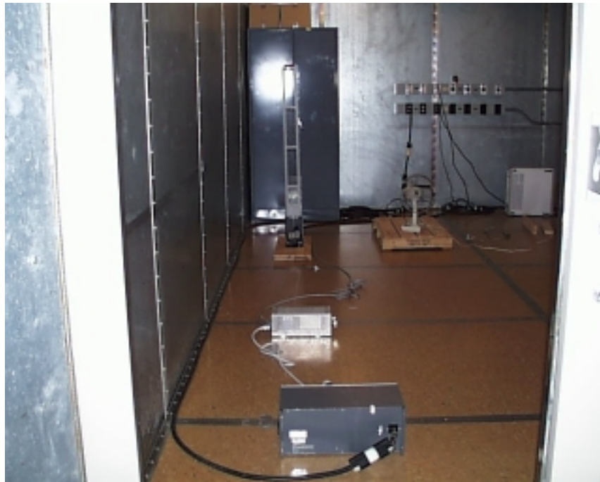
Photo 3 – Photo of Conducted Emission test setup of STRATASX FCC ID D04STRATASX
