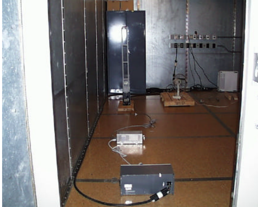
Photo 6 – Strata SX Conducted Emissions Test Setup
