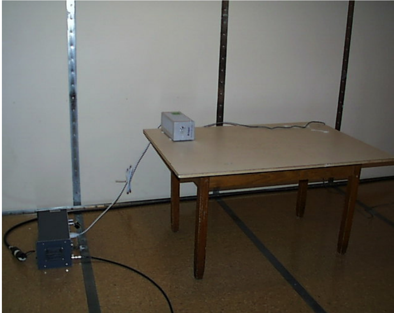
Photo 8 – Strata PX w/TR4024/22 Control Board Conducted Emissions Test Setup
