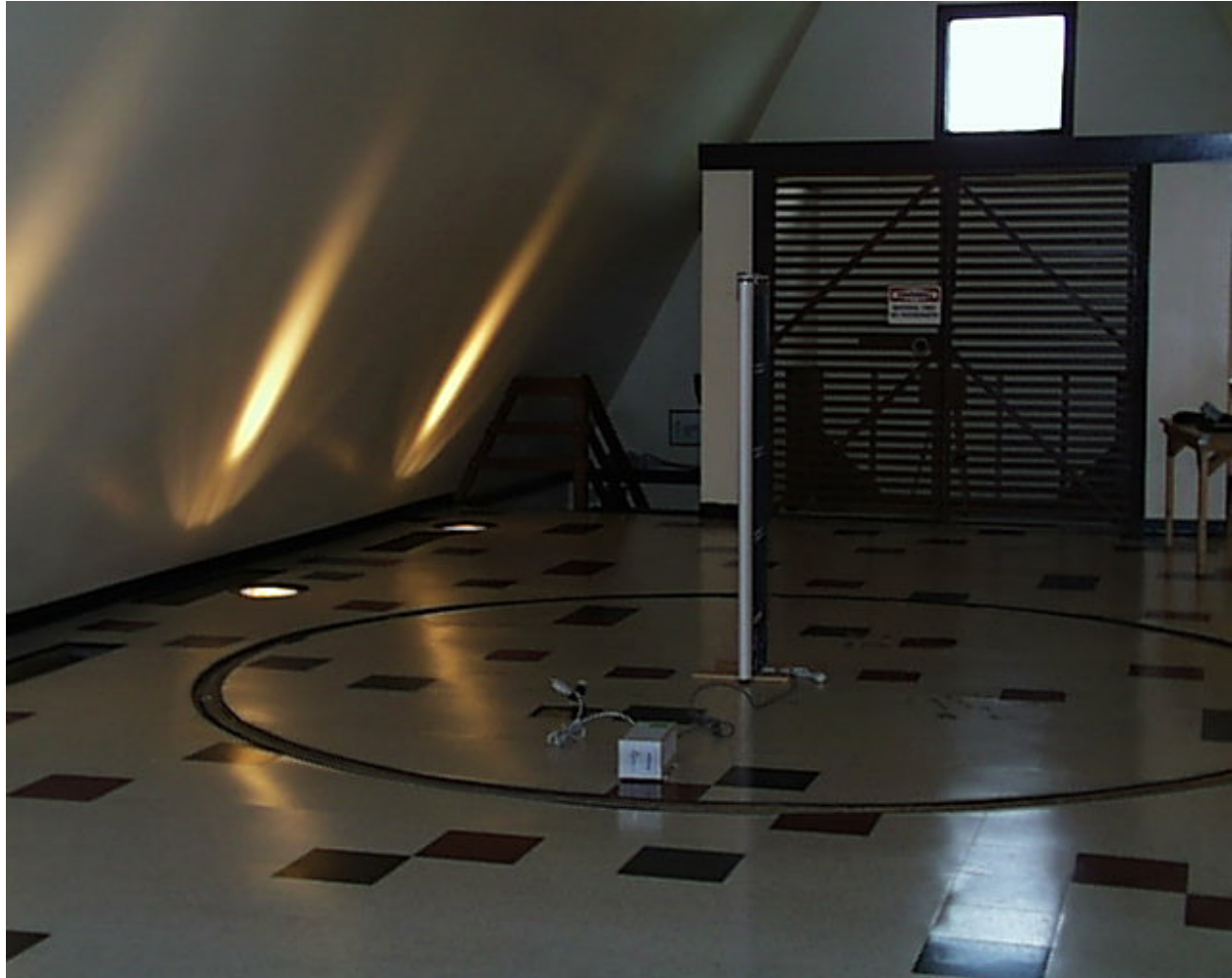
Photo 4 -- Strata PX w/TR4024/22 Control Board Radiated Emissions Test Setup – Rear View
