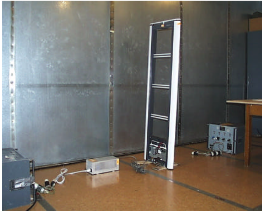
Photo 6 – Strata PX Conducted Emissions Test Setup
