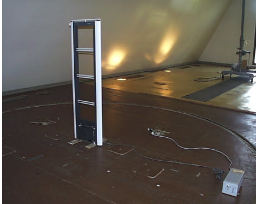
Photo 3 -- Strata PX Radiated Emissions Test Setup – Front View
