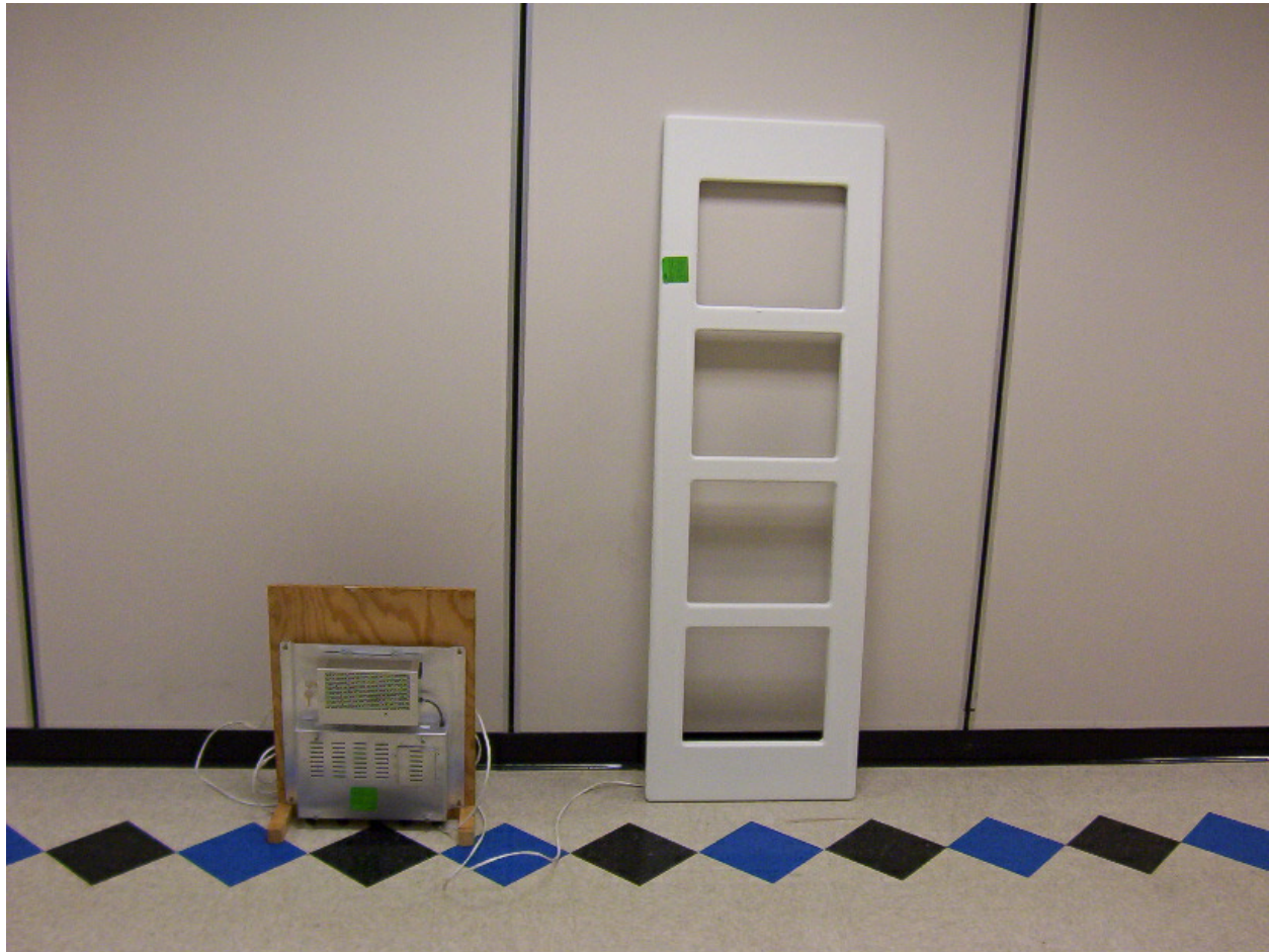
Photo 1 – Image of TR4025 Control Module and Antenna Element of Strata OX
