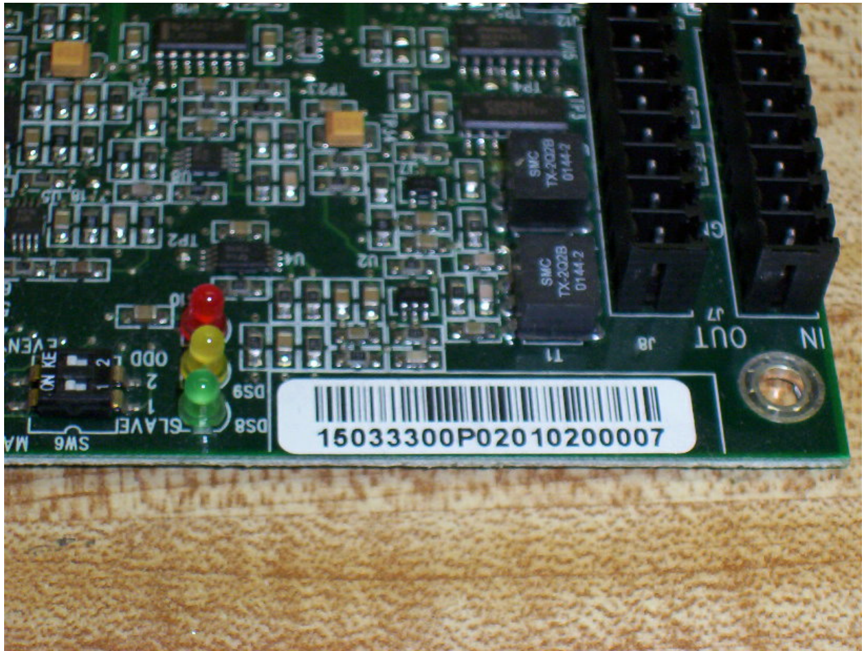
Photo 4 – Serial Number Identification of TR4025 Control PCB
