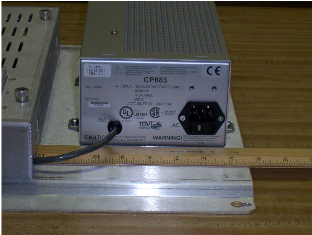
Photo 4 – Power Supply Labeling Information
