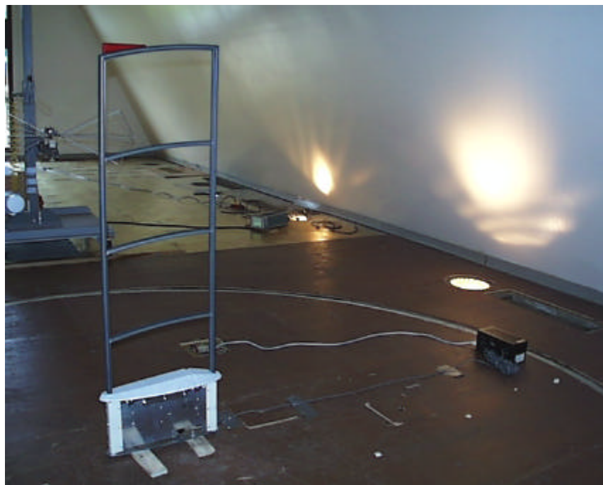
Photo 4 -- Strata MX Radiated Emissions Test Setup – Front View
