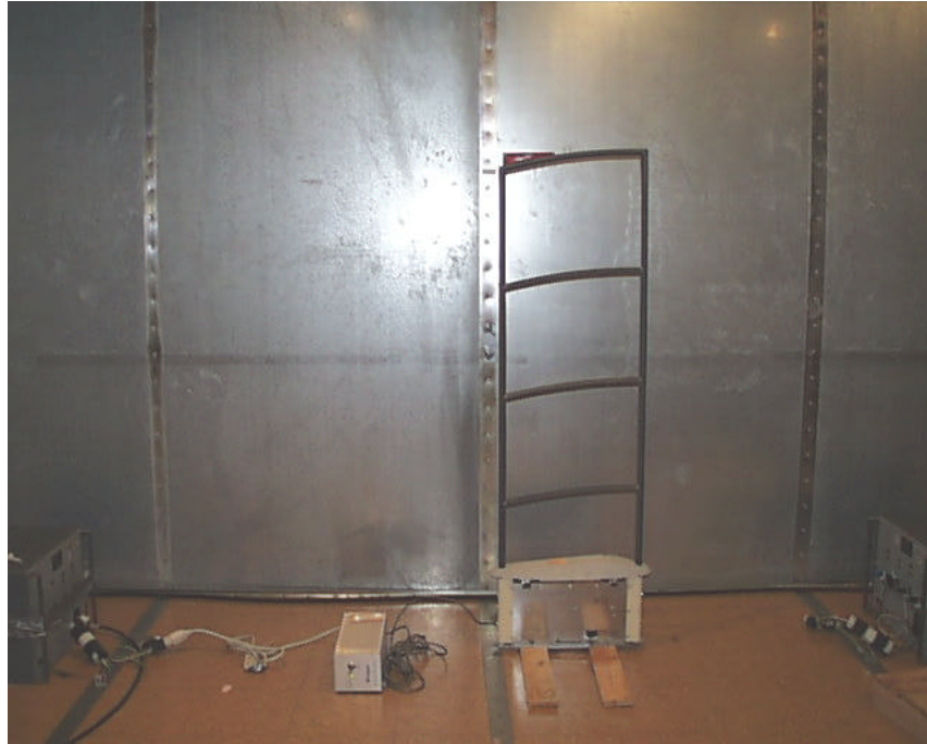
Photo 7 – Strata MX Conducted Emissions Test Setup
