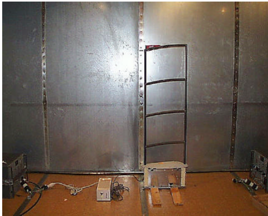
Photo 7 – Strata GX Conducted Emissions Test Setup
