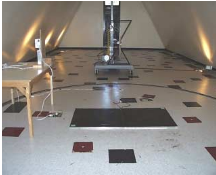
Photo 3 -- Strata FX Radiated Emissions Test Setup – Rear View
