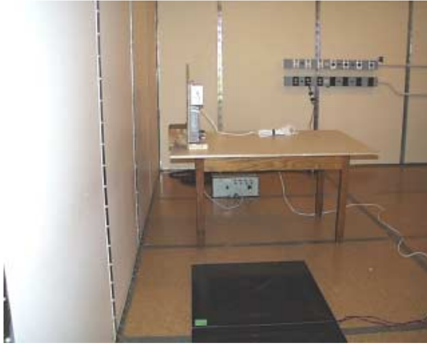
Photo 6 – Strata FX Conducted Emissions Test Setup
