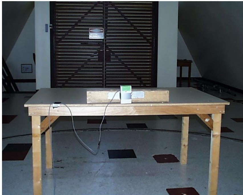
Photo 2 – Performa Switch Plate Radiated Emissions Test Setup - Front
