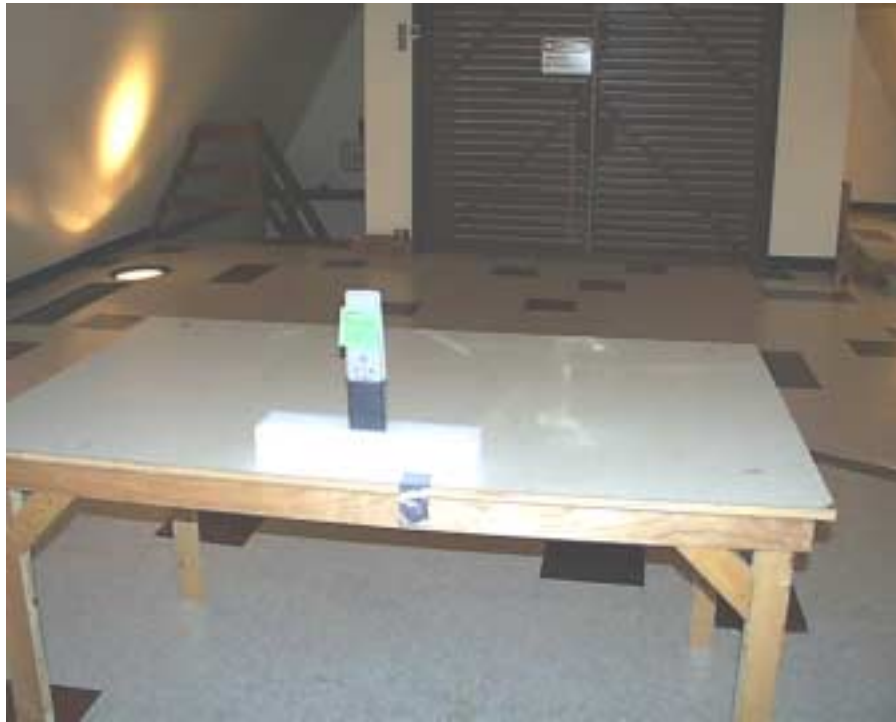
Photo 2 – Portable Verifier Model PV2000 Radiated Emissions Test Setup – Front View
