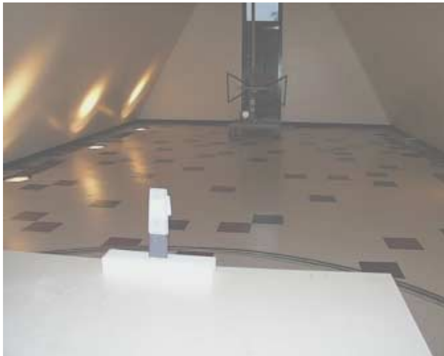
Photo 3 – Portable Verifier Model PV2000 Radiated Emissions Test Setup – Rear View
