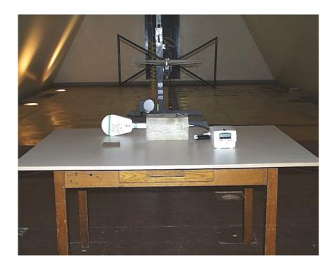
Portable Reader - Radiated EMI Test Setup
